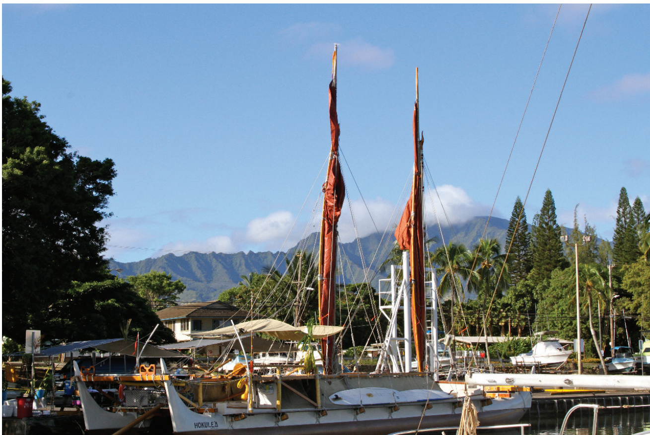
Hokule'a complex Sailing Canoe completed in 1975 has two 62 foot hulls, eight crossbeams and two masts. Photo: Banzai Productions
